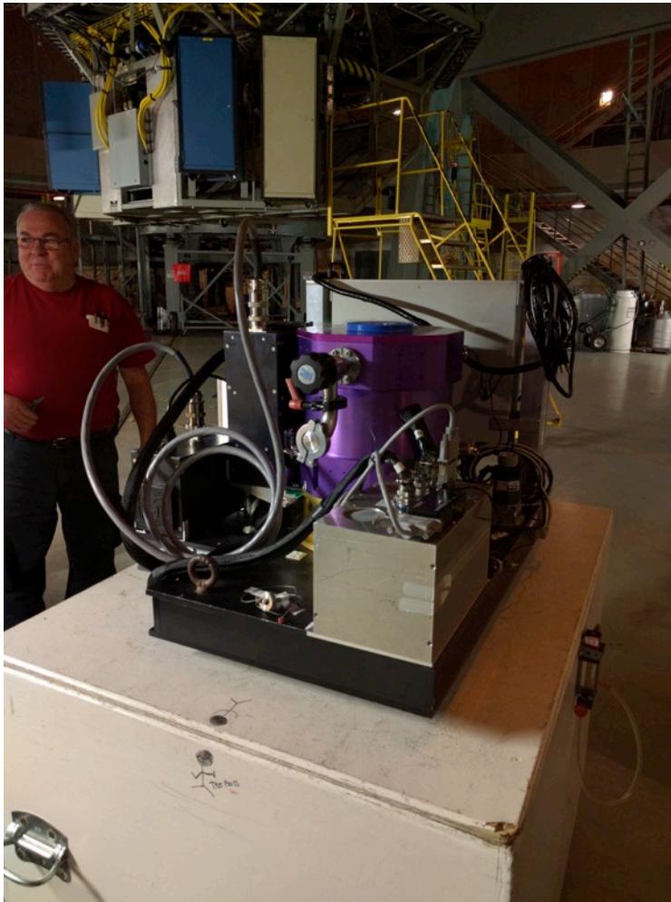
WASP assembled with shutter and filter wheel ready to be lifted to prime focus
